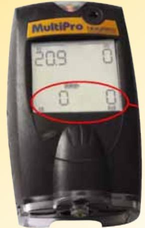
The defect involves the detector's long-term accuracy of carbon monoxide (CO) measurements. When the gas detector is on the CO channel, the sensors exhibit a progressive change in sensitivity, which may lead to the detector under-reporting the true value of CO being measured. This problem may affect any monitor with the duo-tox carbon monoxide/hydrogen sulfide sensor.
